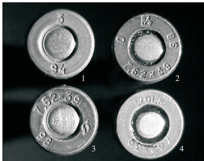
Fig. 1. Representative headstamps on Russian “hunting” cartridges: 1 – Soviet-style headstamp: 3 = Ulyanovsk, 94 = 1994 year of manufacture, bullet = 123 gr JHP-BT with plastic base plug; 2 – Barnaul 125 gr JSP, 1998 manufacture (note symbol at 12 o'clock); 3 – Ulyanovsk 124 gr JHP, 1998 manufacture (note symbol at 4 o'clock); 4 – “WOLF” Tula 122 g. JHP-BT, current (1999–2000) production.
