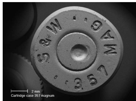
Fig. 9. SEM image of a cartridge case, revealing more depth of focus.
