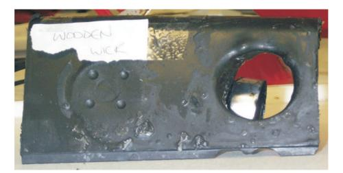
Fig. 4. Ferguson TV casing (after 37 minutes).
