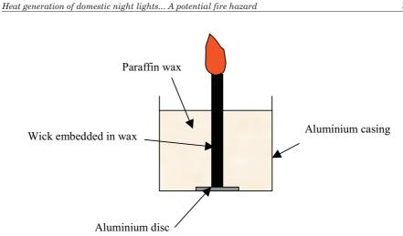
Fig. 1. Components of a typical night light.
