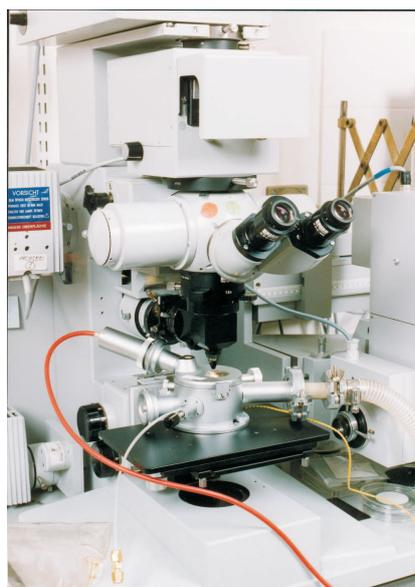
Fig. 6. CL equipment. The basic components are a Leica contrasting unit (with a cold-cathode electron gun) and a microspectrophotometer (Zeiss UMSP 80).
