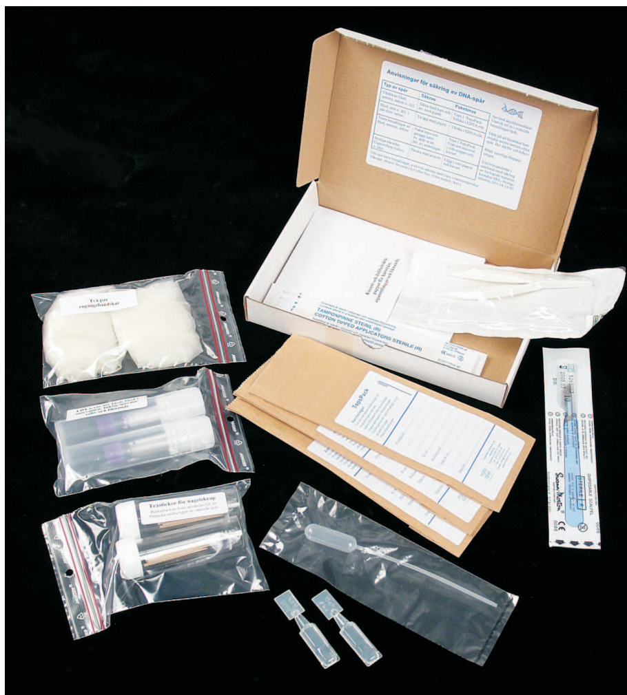
Fig. 1. The Swedish DNA kit contains the following items; Cottons swabs and corresponding “topspacks” (containers), envelopes, water ampoules, a scalpel, a pipette, wooden sticks (dental), glass tubes and a pair of disposable latex gloves. In addition, guidelines for sampling, packaging and further handling of stains to be collected, are printed inside the lid.
