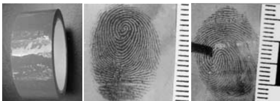
Fig. 3. Fingerprint developed on adhesive side of sticky tapes coated with polyisoprene glue (left – RTX/right – sticky side powder).
