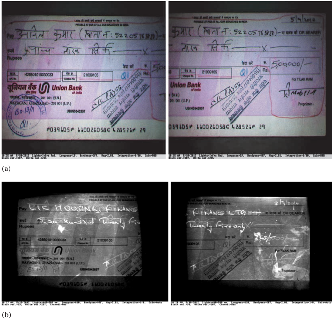
Fig. 6. a) Actual photographs of a bank instrument with writings and signatures executed with normal ink visible to the naked eye; b) processed photographs of the same bank instrument as shown in Figure 6a above, revealing secret writings below the existing writings using a spotlight in the VSC-2000 HR.
