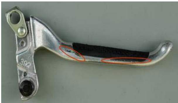
Fig. 1. Smears on brake lever.
