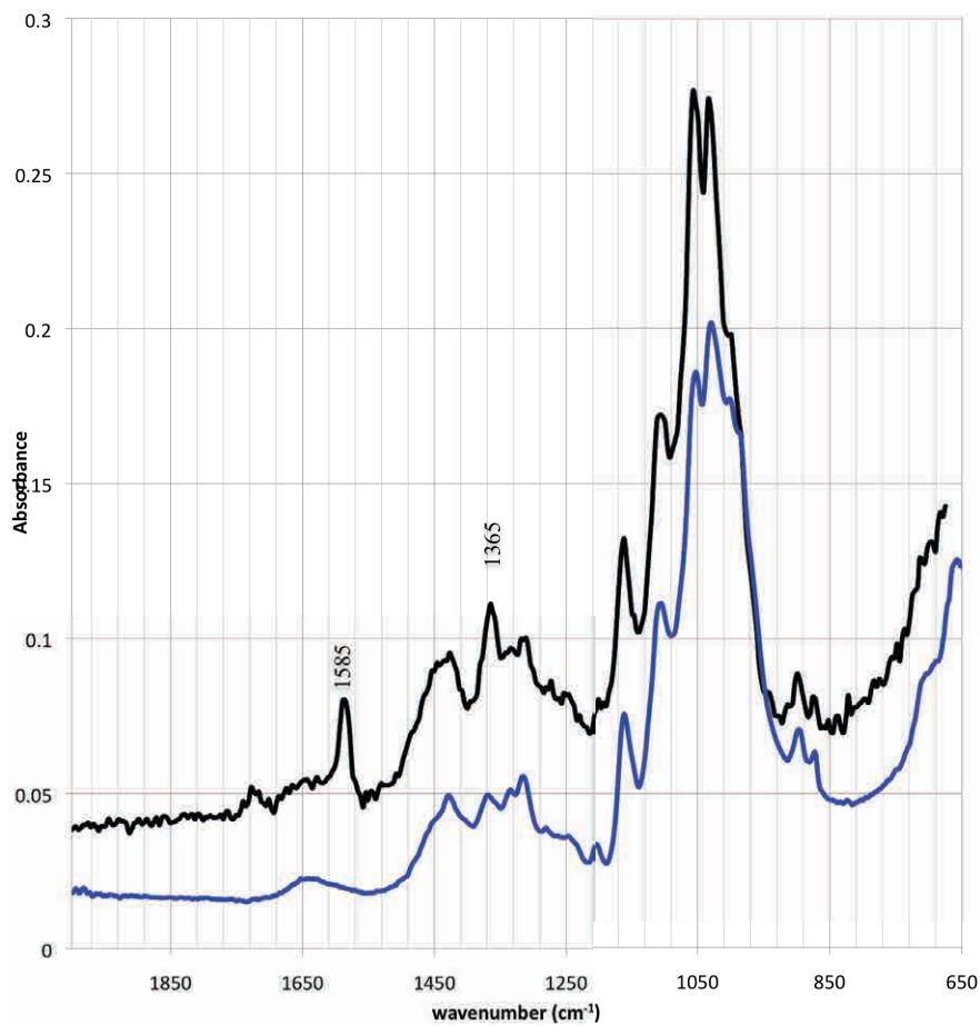
Fig. 1. FTIR spectrum of ink spot (M1) deposited on paper substrate (black line) from 2000 to 675 \text{cm}^{-1} , overlaid by spectrum of blank paper (blue line).
