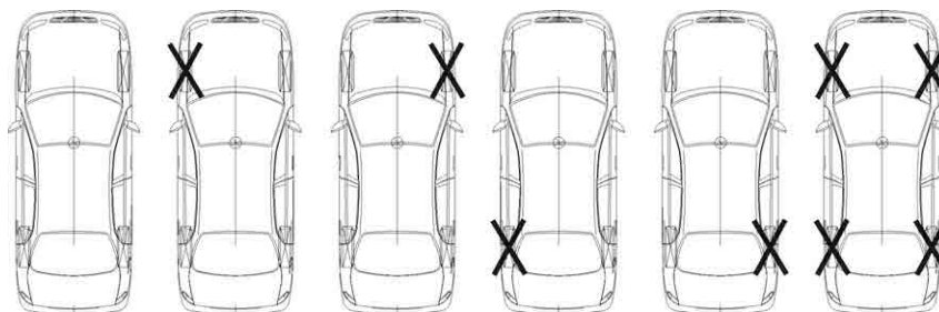
Fig. 3. The order of reduction and elimination of tire pressure.
