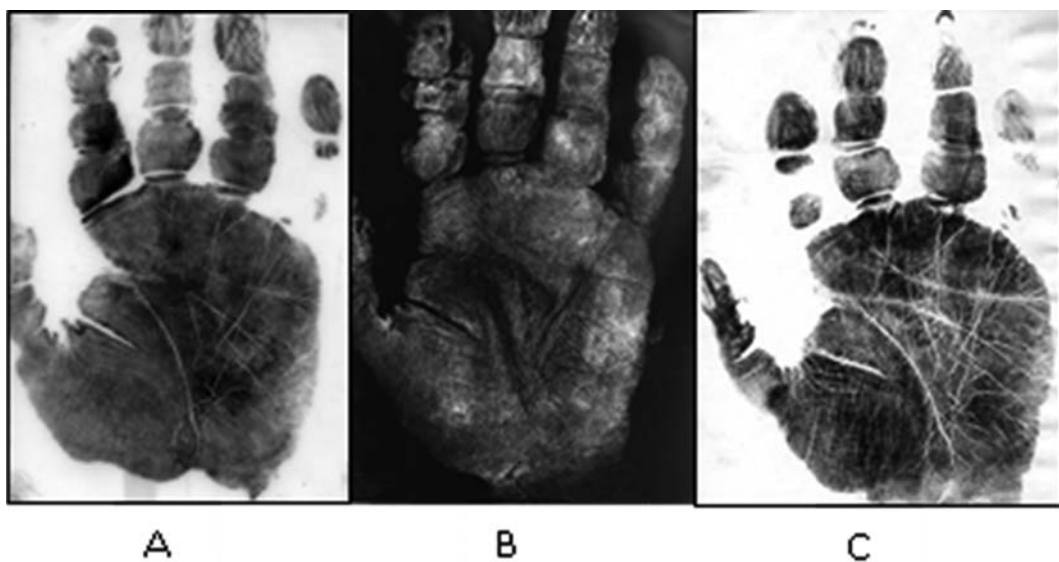
Fig. 2. Cheirosopic prints executed after dusting with black powder (A), aluminium powder (B), and ink (C).
