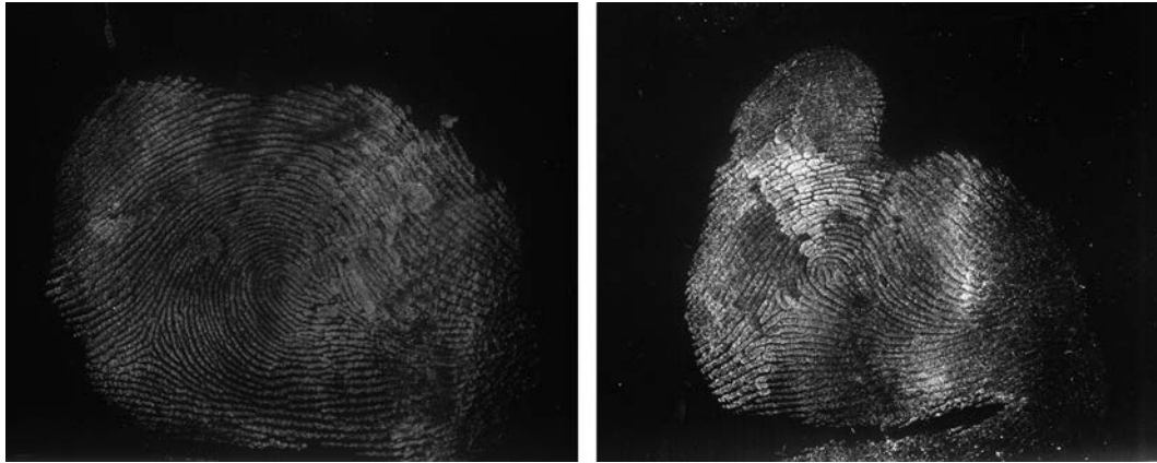
Fig. 4b. Powder prints on fingerprint lifter after previously rubbing glycerol cream into fingertips.
