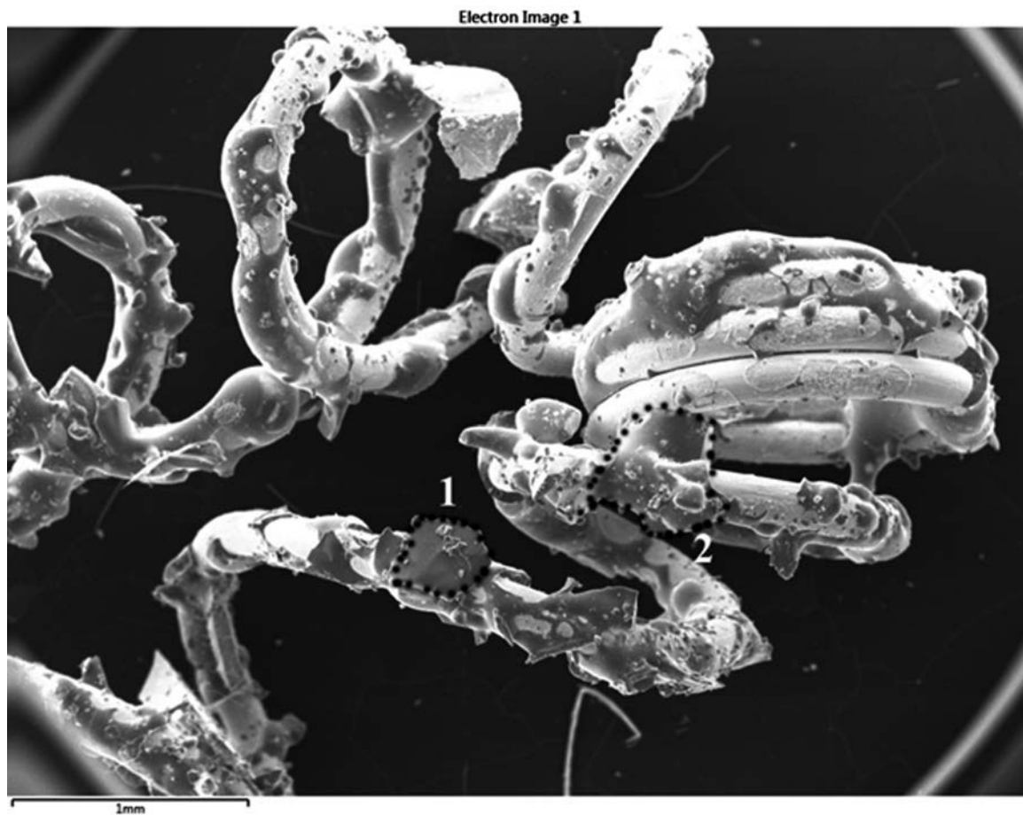
Fig. 2. The filament of the bulb with glass melted onto the filament – observed with the use of a scanning electron microscope. (1) and (2) denote sites at which the elemental composition was analysed.
