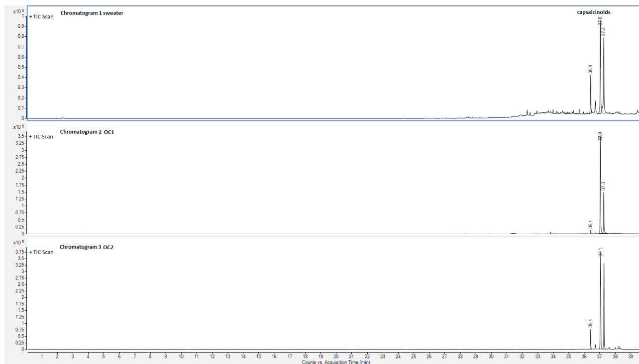
Fig. 10. Chromatograms obtained by the injection of the extract from the sweater (Chromatogram 1), preparation from the first pepper spray, marked as OC1 (Chromatogram 2) and preparation from the second pepper spray, marked as OC2 (Chromatogram 3).
