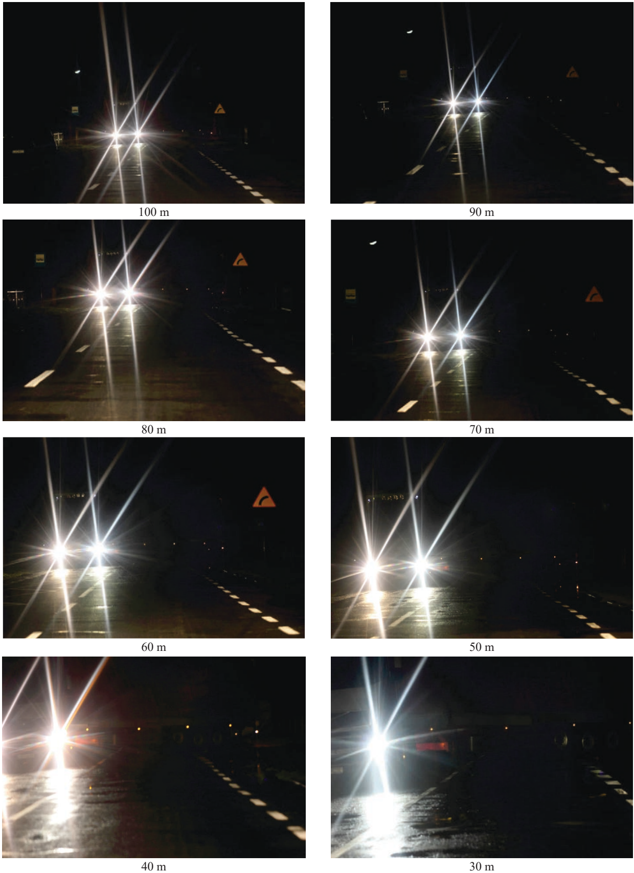
Fig. 16. Stopped combination vehicle from subsequent distances from 100 m to 10 m from the semitrailer, every 10 m.
