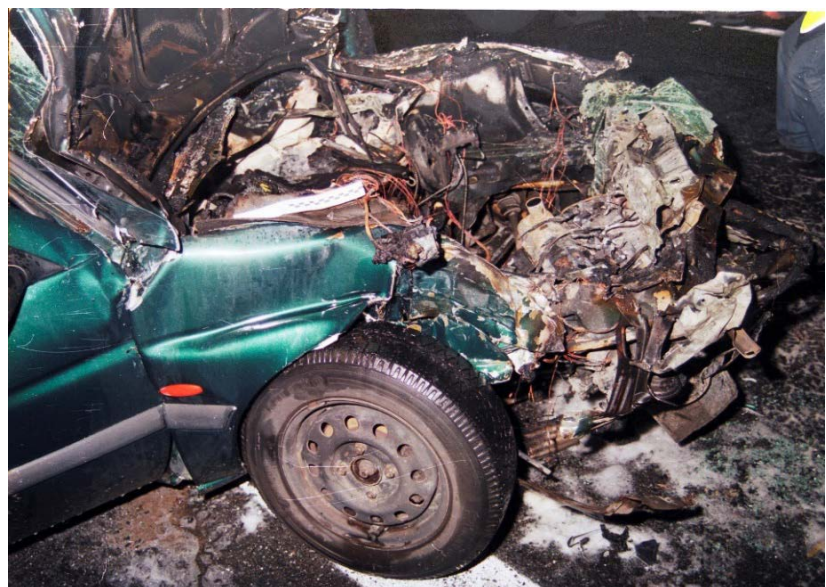
Fig. 7. Deformation of the Ford's engine compartment.
