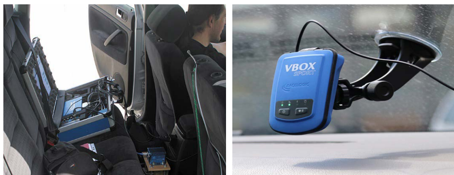
Fig. 2. VBox measurement apparatus fixed in the Volkswagen car – photographs by the authors.
