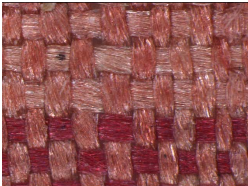
Fig. 7. Image from a stereoscopic microscope of a fragment of external fabric of the cushion labelled evidence no. 1.
