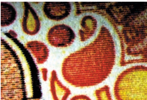
Fig. 7. Microscopic examination of colored xerographic documents shows the presence of colored toner particles, i.e., cyan, magenta and yellow, and black colour. The characters are in half-toned mode and the toner particles are deposited on the surface of the paper and the edges of the characters are distorted.
