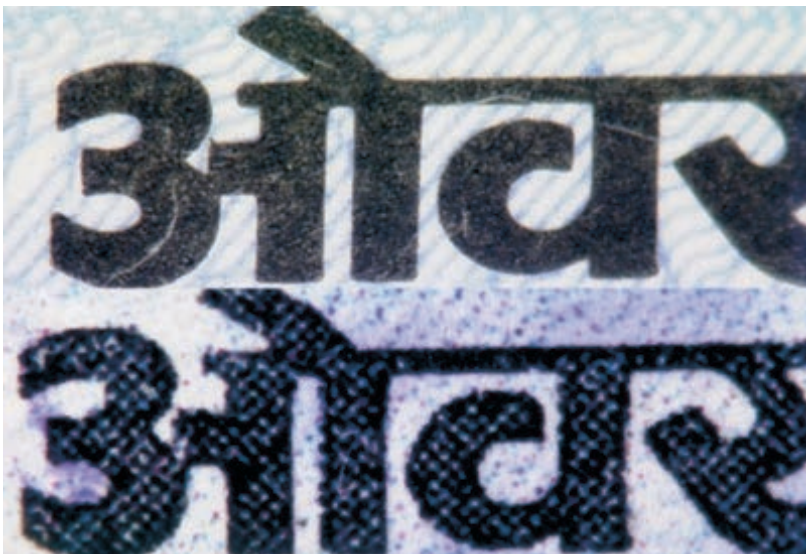
Fig. 10. Magnified upper sample image is offset lithography as indicated by clear lines and even printing while lower disputed image is scanned copy of upper offset image and printed by laser printer as shown by the presence of symmetrical arranged coloured toner particles in the characters and the background.
