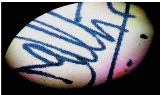
Fig. 5a. The stereo-microscopic image of signature as shown in the Fig. 5, reveals that the strokes of signature are comprised of different coloured (cyan, magenta, yellow) array of dots of toner particles indicating that the signature is not a manuscript but reproduce mechanically using colour laser printer.
