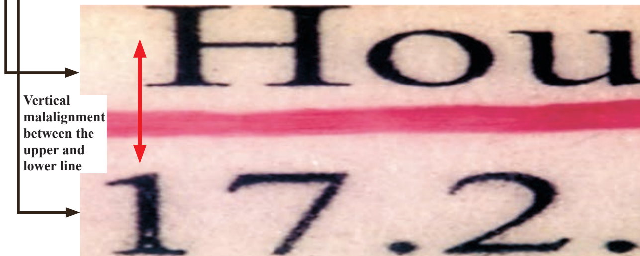
Fig. 3a. Under microscopic examination of the disputed cash receipt as shown in above Fig. 3, it is observed that there are changes in the appearance (shining) of the printed characters. On careful observation of matrix of the characters, deposition of toner particles in the periphery of the figures “17.2.” observed whereas there is no such deposition of toner in the periphery of upper word “Hou” indicating that the disputed texts in the lower line was carefully interpolated using different printer.
